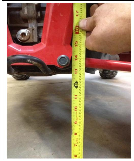
$\frac{1}{2}$ " more ride height you should lower the collar about  $\frac{1}{4}$ ". The rear should be about  $\frac{1}{2}$ " lower than the front or 16" of ground clearance. This is measured in the rear, center of the RZR, from the bottom of the chassis to the ground just below the rear tow hook. Always drive the RZR between adjustments. You are done!
